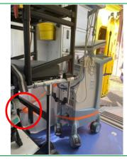
Pass the strap through the black D-ring seen in bottom left of photo. Ensure the strap is around the base the of unit and not around the wheels.
