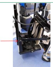
Unscrew the grey cap and lift support arm
