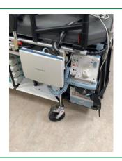
Place the display monitor onto the round mount on the side of the trolley, once mounted the screen can be opened
