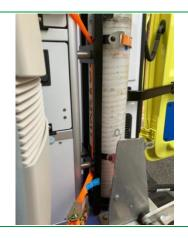
The strap must pass through the black oyygen holder as this is bolted to the ambulance chassis
